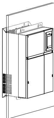
Figure 3-11 Embedded installation effect of the SVD-P (sheet metal housing)
